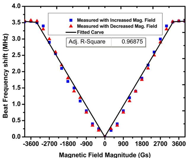
Fig. 4. The measure beat frequency shift of the fiber laser for various applied magnetic field magnitudes. A fitted curve for the measured results is also plotted as the solid line.
