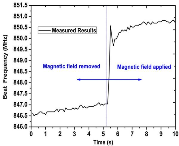
Fig. 3. Measured beat frequency when a 3600 Gs magnetic field is applied to the fabricated fiber-optic magnetic field sensor.
