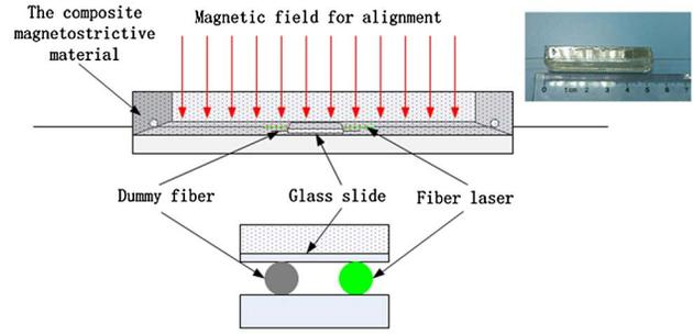
Fig. 1. The fabricated fiber-optic magnetic field sensor created by embedding a heterodyning fiber laser into an epoxy resin-bonded magnetostrictive composite material with Terfenol-D particles incorporated.
