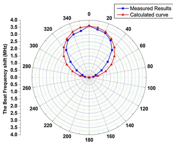
Fig. 6. The beat frequency shift of the fiber laser for various angles between the sensor and magnetic field direction with a 3600 Gs magnetic field applied. A calculated curve is also plotted as the solid line.
