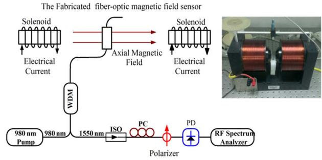
Fig. 2. The experimental setup for the magnetic field measurement. ISO: isolator; WDM: wavelength division multiplexer; PC: polarization controller; PD: photo detector.
