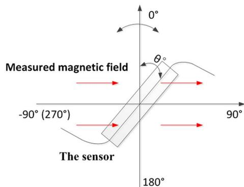
Fig. 5. The setup to measure the directivity of the proposed fiber-optic magnetic field sensor. The direction of the measured magnetic field is fixed, but the direction of the sensor is rotated to different angles.
